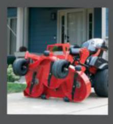
THE MAINTENANCE-FRIENDLY, STAND-UP DECK allows you access to the blades quickly and easily. Need to untangle something? Just flip the deck, fish out your dog's pull toy and get back to mowing
